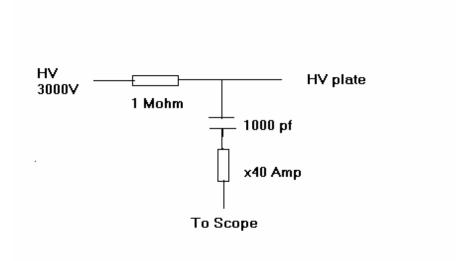
The micro-discharge signal is taken directly from the HV feed through a 1000 pF capacitor. The capacitor is rated for 7kV. The signal is amplified by 40 times and connected to a Lecroy Digital Scope to record the pulse shape. The HV applied to the plate is 3000 volts.
