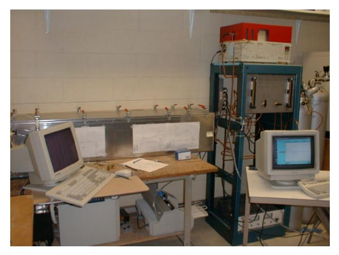
The dimension of the box (made of aluminum and sitting on the long table in the picture above) are 30 cm x 30 cm x 170 cm. The box was designed to accommodate the largest module (type III). For type II, about 1/3 of the space inside is filled with ballast material to reduce the overall volume. The GC (red color) is sitting on the top of the rack in the picture.
