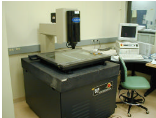
Figure 1 Photograph of the OGP Avant-600 non-contact optical measuring machine used to measure the Barrel TRT HV plates prior lamination of the kapton HV distribution circuit. It has measurement area of 18"x24" and measurement accuracy of \pm 0.005\text{mm}
