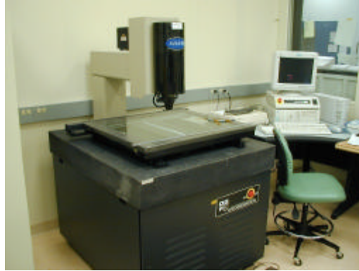
Figure 1 Photograph of the OGP Avant-600 non-contact optical measuring machine used to measure the Barrel TRT tension plates .It has measurement area of 18"x24" and measurement accuracy of \pm 0.005\text{mm} .
