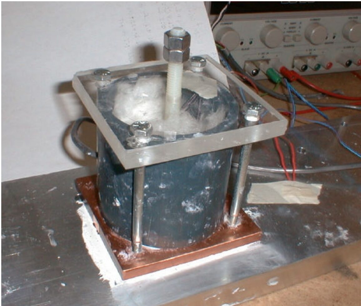
Figure 2 – This photograph shows the assembled thermal conductivity test setup. The gray cylinder and white insulation surround the copper heater cylinder and epoxy sample shown in figure 1.
