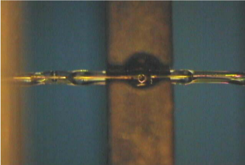
Figure 1. A picture of a wire-joint still in a production jig. One can see two melted regions and the center melt, and wire. The length is \sim 5\text{-}6 mm.
