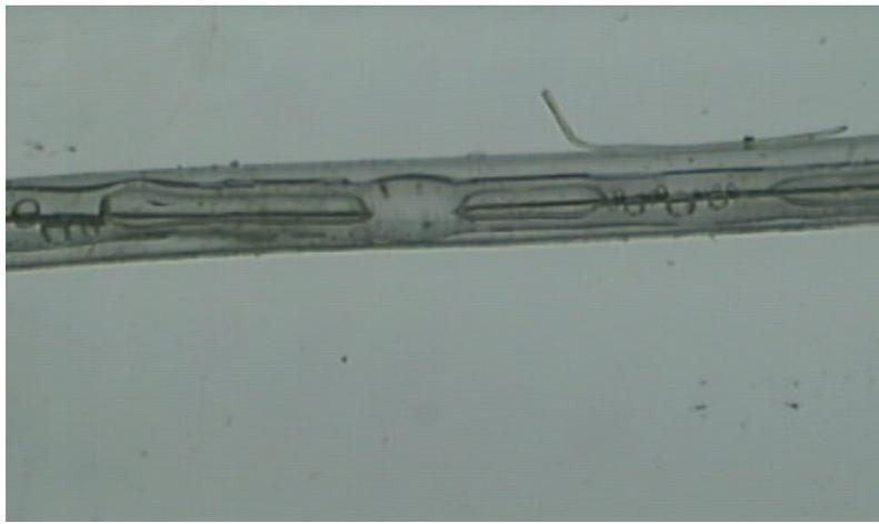
Figure 2. Encapsulated glass wire-joint after the radiation. Shown is the middle part of the wire-joint. This was in Xe-CO<sub>2</sub> gas mixture.
