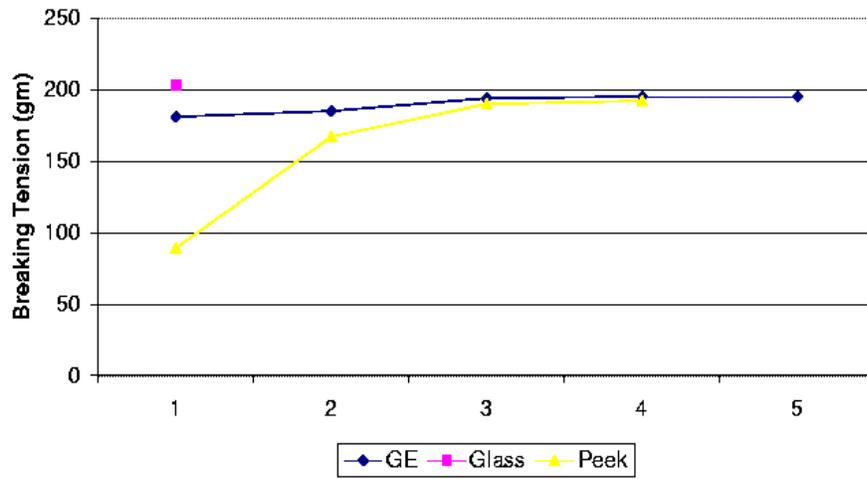
Figure 6. The tension when a wire segment with wire-joint fails. When the breaking tension is near 200 grams, the failure mode is the broken wire rather than the wire-joint failure.
