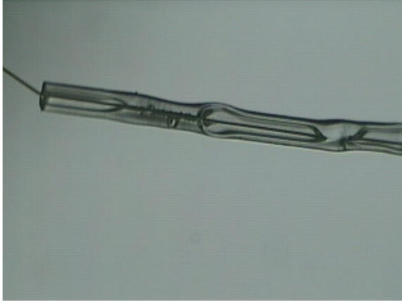
Figure 1. Glass wire-joint after ~1 C/cm radiation. This was in Xe-CO<sub>2</sub> gas mixture.
