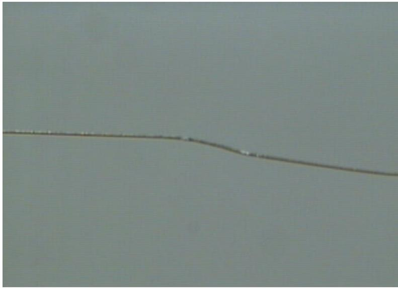
Figure 5. A picture of wire with gold etched away. This was in Xe-CF<sub>4</sub>-CO<sub>2</sub> gas volume.
