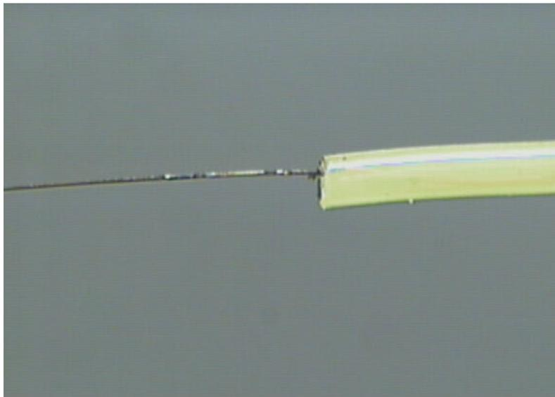
Figure 4. Peek wire-joint after the radiation. This was in Xe-CF<sub>4</sub>-CO<sub>2</sub> gas volume.
