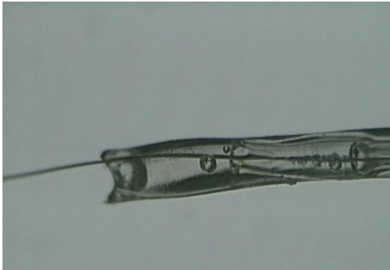
Figure 3. Encapsulated glass wire-joint after the radiation. This was in Xe-CF<sub>4</sub>-CO<sub>2</sub> gas volume.
