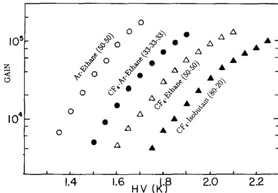
Fig. 12. The gain as a function of high voltage for several gas mixtures.
