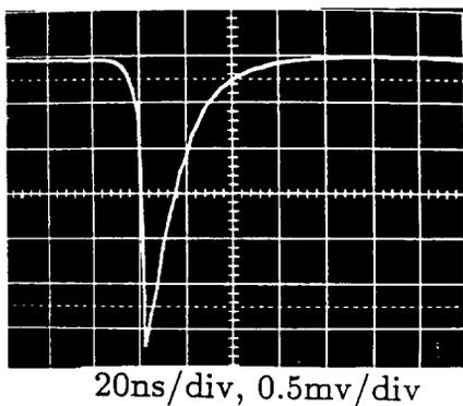
Fig. 9. The averaged signal using  $^{90}\text{Sr}$  source. The gas mixture is  $\text{CF}_4$ -Ar-ethane (33-33-33) and high voltage is 1800 V.
