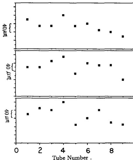
Fig. 7. Horizontal position of straw tubes in the third layer as a function of straw tube number. The plotted points are the difference between the measured position and the expected position with respect to the first tube. Each plot is taken at a different distance from one end along the length of tubes. The measurement error in each point is about 25  $\mu\text{m}$ .
