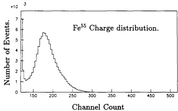
Fig. 13. Typical  $^{55}\text{Fe}$  spectrum measured from a cell using a multichannel analyzer.
