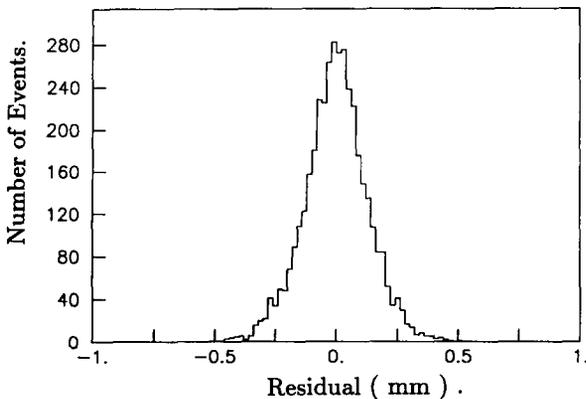
Fig. 16. Residual in mm obtained using cosmic ray tracks. Only tracks with six or more hits are used. Sigma of  $110 \mu\text{m}$  obtained from a Gaussian fit to the curve.
