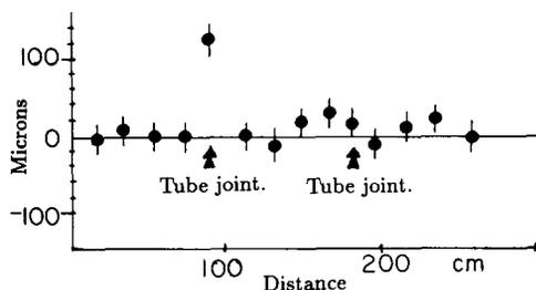
Fig. 8. The vertical position of straw tubes on the top layer as a function of distance from one end.
