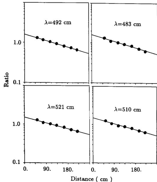
Fig. 11. The ratio of amplitude from one end to the other end using  $^{55}\text{Fe}$  source. The attenuation length is obtained from the slope. See text for detail.
