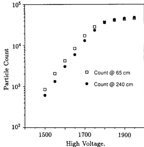
Fig. 10. Plateau curves obtained using  $^{90}\text{Sr}$  source at two different positions from the end of tubes. The gas mixture is  $\text{CF}_4$ -Ar-ethane (33-33-33).
