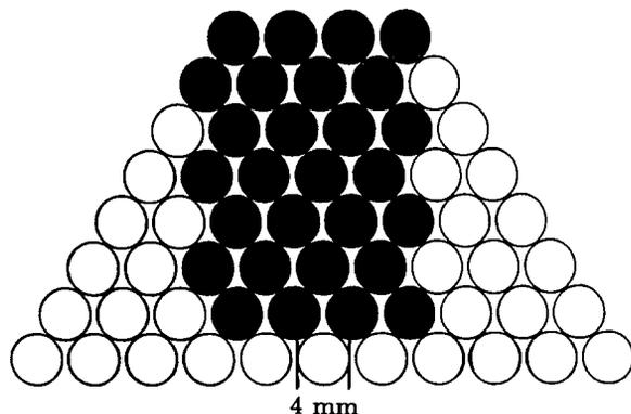
Fig. 4. Cross section of the straw tube superlayer in the prototype. The shaded tubes were instrumented.
