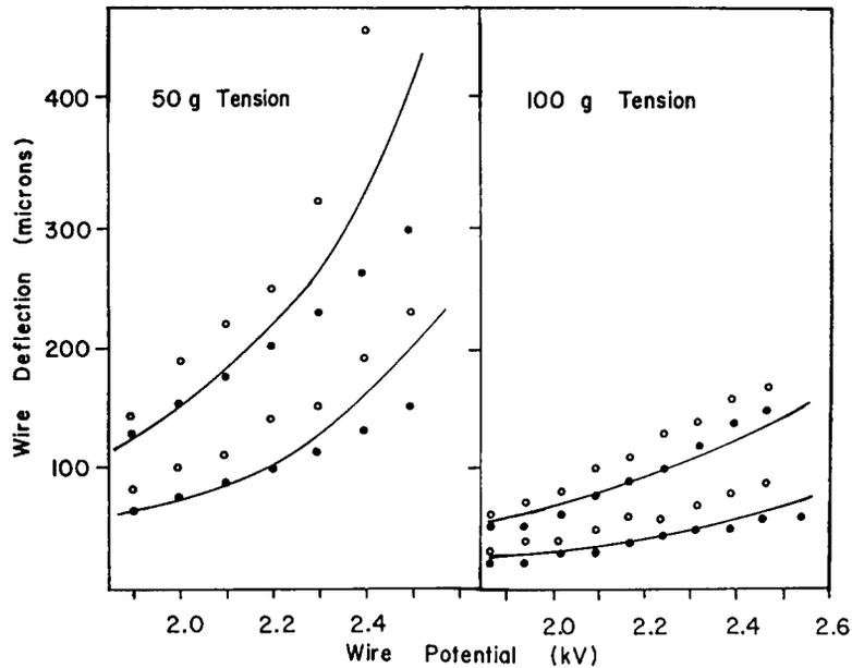
Fig. 2. Wire deflection as a function of voltage for two different initial displacements, 100 (lower set) and 200 (upper set)  $\mu\text{m}$ . The left panel is for 50 g tension, and the right panel for 100 g tension. The solid curves are the prediction from the formula in text. The open circle data points are for initial offset in one direction while the closed data points are for initial offset in the opposite direction.
