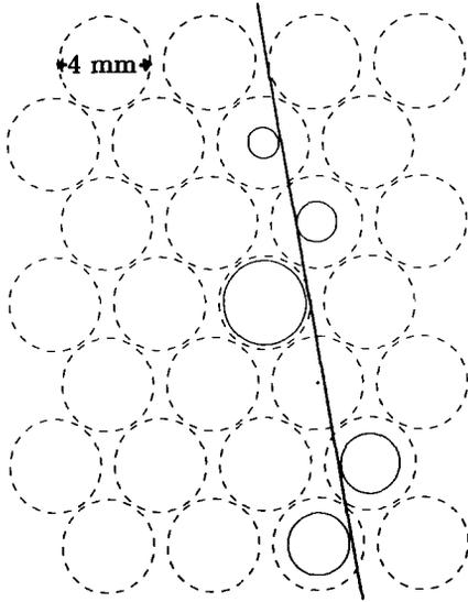
Fig. 15. A triggered cosmic ray track traversing the superlayer.
