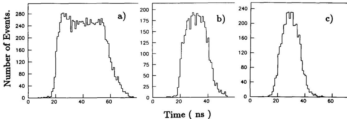
Fig. 14. Raw time distributions measured using different gas mixtures: (a) Ar–ethane (50–50), (b)  $\text{CF}_4$ –ethane (50–50), (c)  $\text{CF}_4$ –isobutane (80–20).
