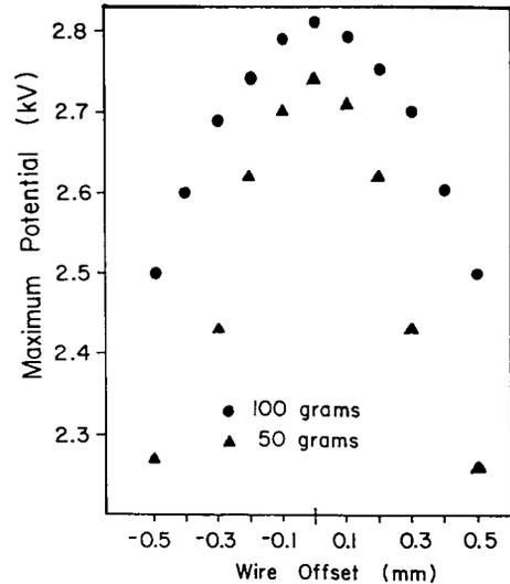
Fig. 1. Maximum stable operating voltage for two different wire tensions of 50 and 100 g as a function of initial wire offset.
