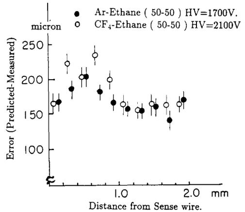
Fig. 17. The error as a function of distance from the sense wire. See the text for the definition of the error.
