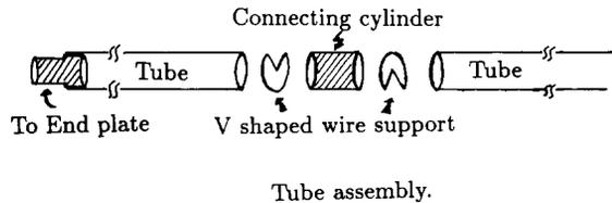
Fig. 5. Tube assembly with tube connector and wire support.
