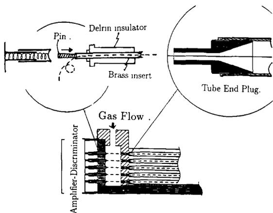
Fig. 6. The endplate used in the prototype. The details of the tube end plug and feedthrough are shown.
