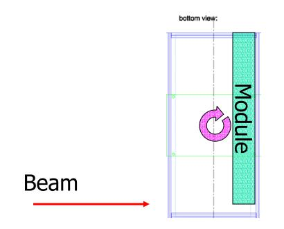
Module motion - rotation in plane of module
