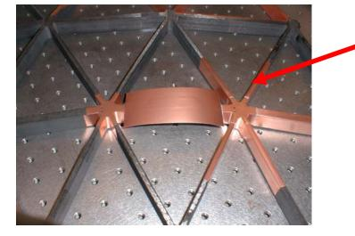
Step 4 – seal tape edges w/ Structural epoxy (silver epoxy shown) Step 3 – Add tape to sides – covering existing pieces
